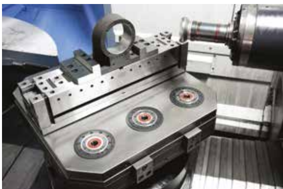
Morsa FMS montata su piastra Zero Point FMS vises mounted on Zero Point plates
